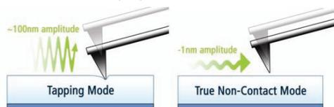
in non-contact mode without damaging the tip or sample. With proper Z-Servo performance, the ultimate resolution of AFM can be achieved in True Non-Contact mode by keeping a constant tip-sample distance of a few nanometers.
