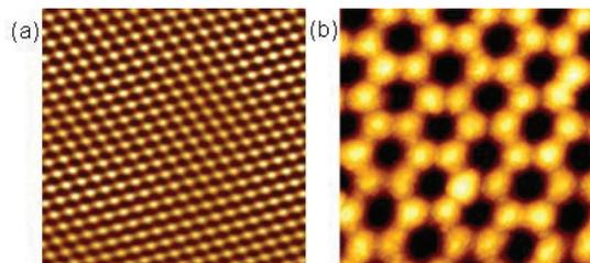
(a) AFM image of HOPG taken with XE-100 (5  $\mu\text{m}$  scan size). This image shows atomic lattice, not individual atoms.
